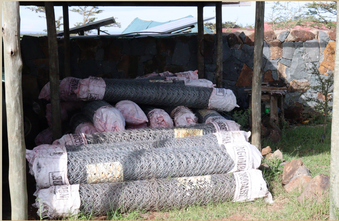
Figure 14: Triple twist chain-links procured to support boma reinforcement efforts in the identified conflict hotspots.
